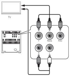
Connect a progressive scan TV through component video cables for higher quality video.
